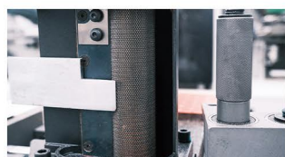
Servo Gluing Unit and Servo Controlled Pressure Rollers
